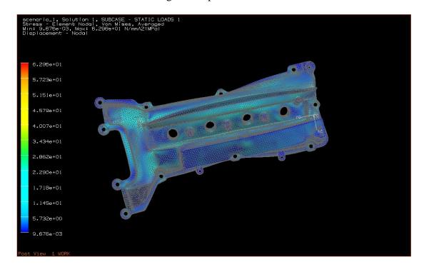
Figure 4 – Engine CAM cover stress distribution (magnesium)
