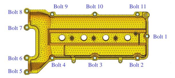
Figure 3 – the cam cover FEA model
