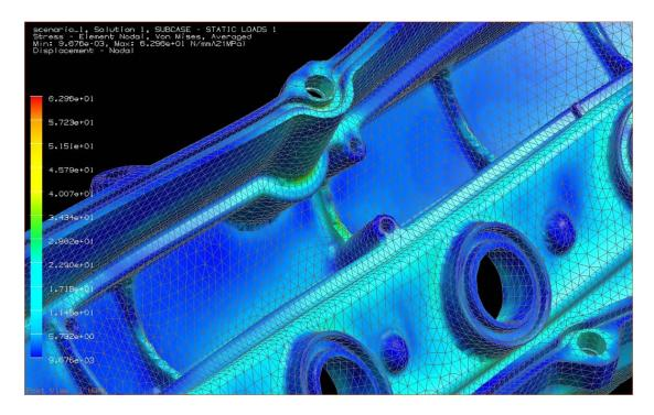
Figure 5 – Engine CAM cover stress distribution zoomed in (magnesium)
