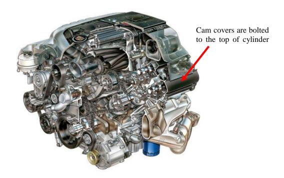
Figure 2 – Engine cam cover
