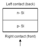
**Figure 1**: Schematic of silicon solar cell with the arrow indicating the direction of light.
