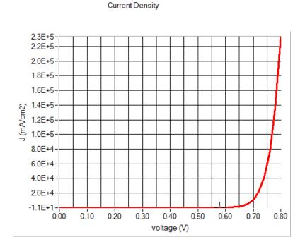
Figure 9: I-V curve of the solar cell under illumination exported from SCAPS.
