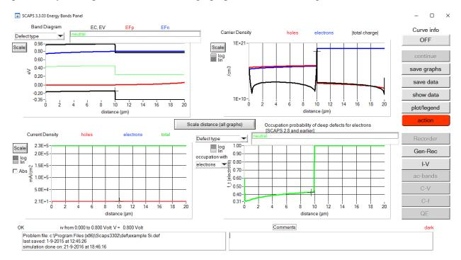
Figure 7: Screenshot of Energy Bands Panel window for the Si cell design.
