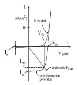
Figure 9: Parameters for calculating the efficiency of the solar cell
