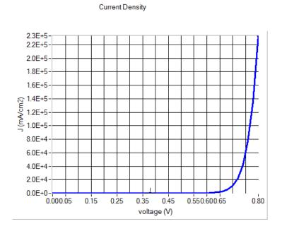
Figure 8: I-V curve of the solar cell under darkness exported from SCAPS.
