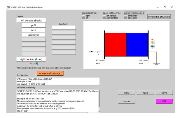
Figure 6: Solar Cell Definition Panel for Si solar cell.
