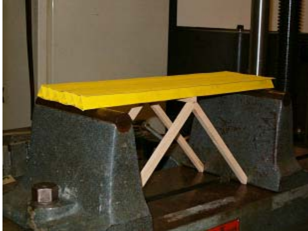
Figure 5. Model arch bridge. Caption: This model bridge is supported at each end and in the center. The center support is a simple arch.
