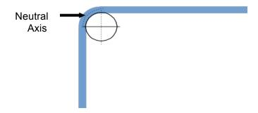
The radius to the neutral axis is our Bend Radius + ½ Material Thickness. (BR + ½ MT)
