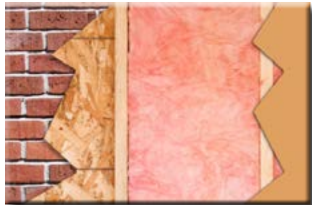
Figure 1: Insulated wall consisting of (from outside in); brick, plywood, 2X6 framing, fiberglass insulation, and drywall
